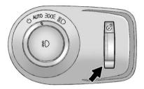
This feature controls the brightness of the instrument panel lights.
